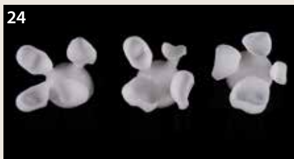
Fig. 24: Press results after divesting with glass beads.
